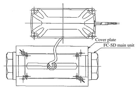
3. Remove the two screws that secure the cover plate diagonally.
