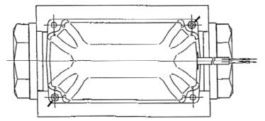
2. Push the cable inside the cover case and, while maintaining enough room, remove the case.
