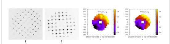
Examples of wavefront sensor images (left) and estimated optical wavefronts from the images (right). The sensor images are analyzed with your own code to estimate the distorted wavefront.
