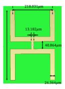
2-1. CST: this is powerful tool to simulate the performance of the detector chip antenna. This tool is used to optimize the antenna attached to the detector in microwave region.
