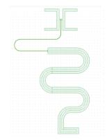
2-3. Sonnet: This tool is used to simulate resonance frequency of the designed resonator circuit. Example is kind of superconducting microwave detector MKID.
