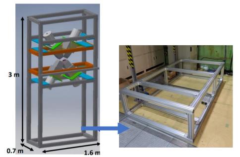
Assembling the frame of Ge detectors.
