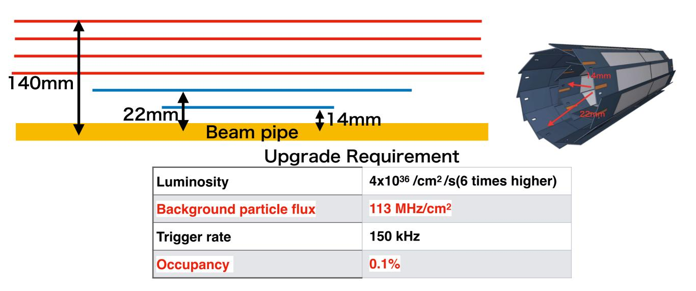
Upgraded SuperKEKB luminosity will be 6 times larger than now, it will make a tough background environment for PXD to reconstruct track. Development of next PXD need to consider these background challenge. KEK SOPIX group develops a pixel detector for Belle II upgrade PXD.
