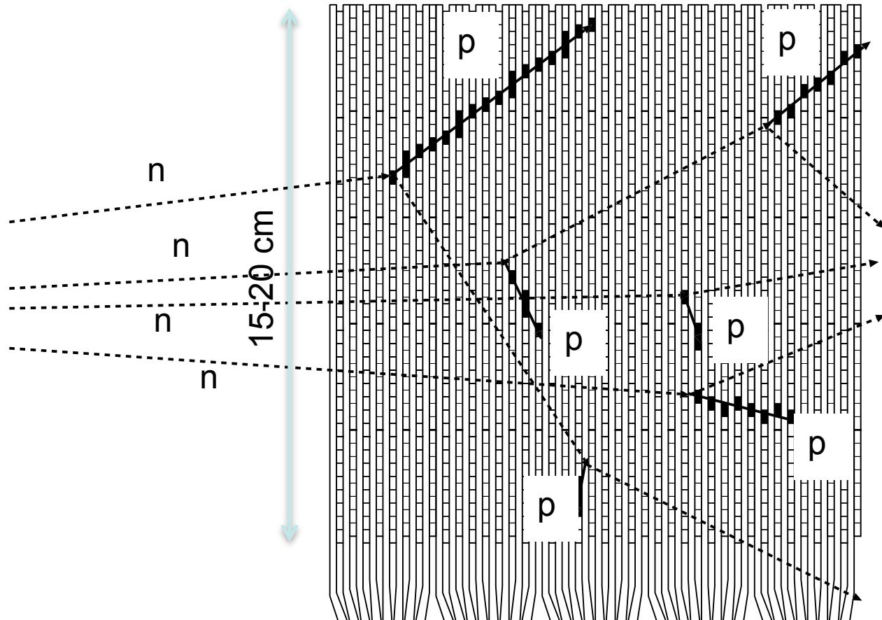
Micro-Hodoscope:  $2.5 \times 5 \text{ mm}^2$
