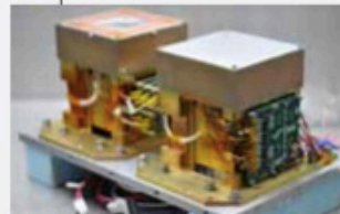
X-ray sensor and signal-processing electronics
