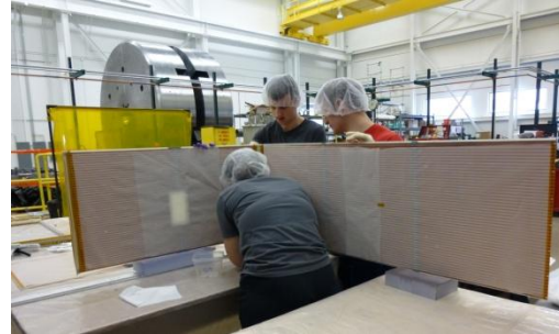
Gluing field cage together
