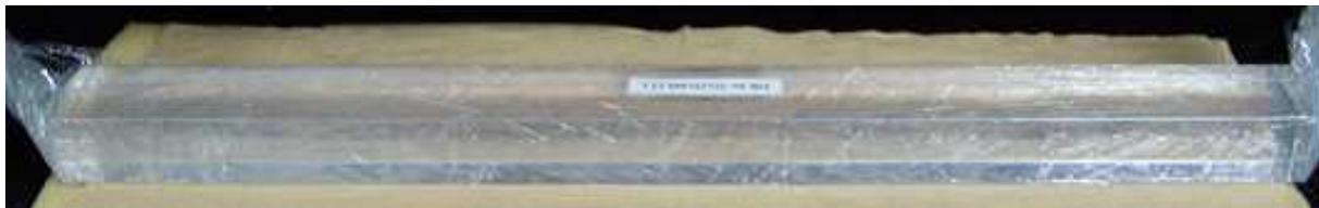
Figure 3.10: A picture of BGO crystal, whose size is  $30 \times 25 \times 400 \text{ mm}^3$ , for scintillation calorimeter.
