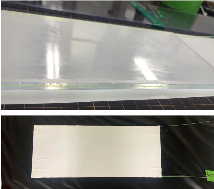
Figure 4.1: Process of embedding wavelength shifting fibers in a groove on the scintillator slab, fixing them with optical cement (top) and wrapping the slab with Teflon sheet (bottom).
