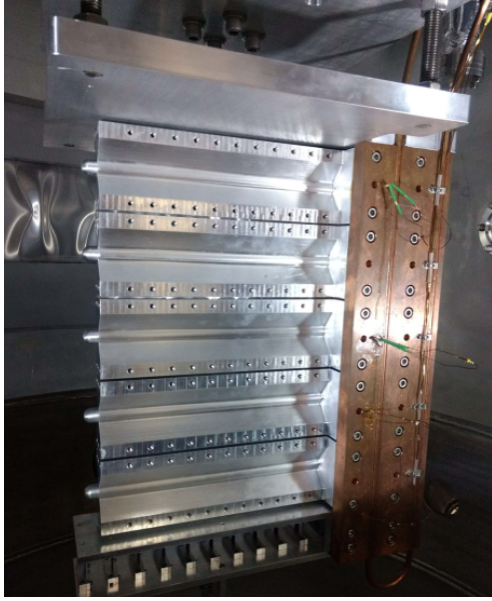
Figure 3.6: A photo of the target system into the vacuum chamber
