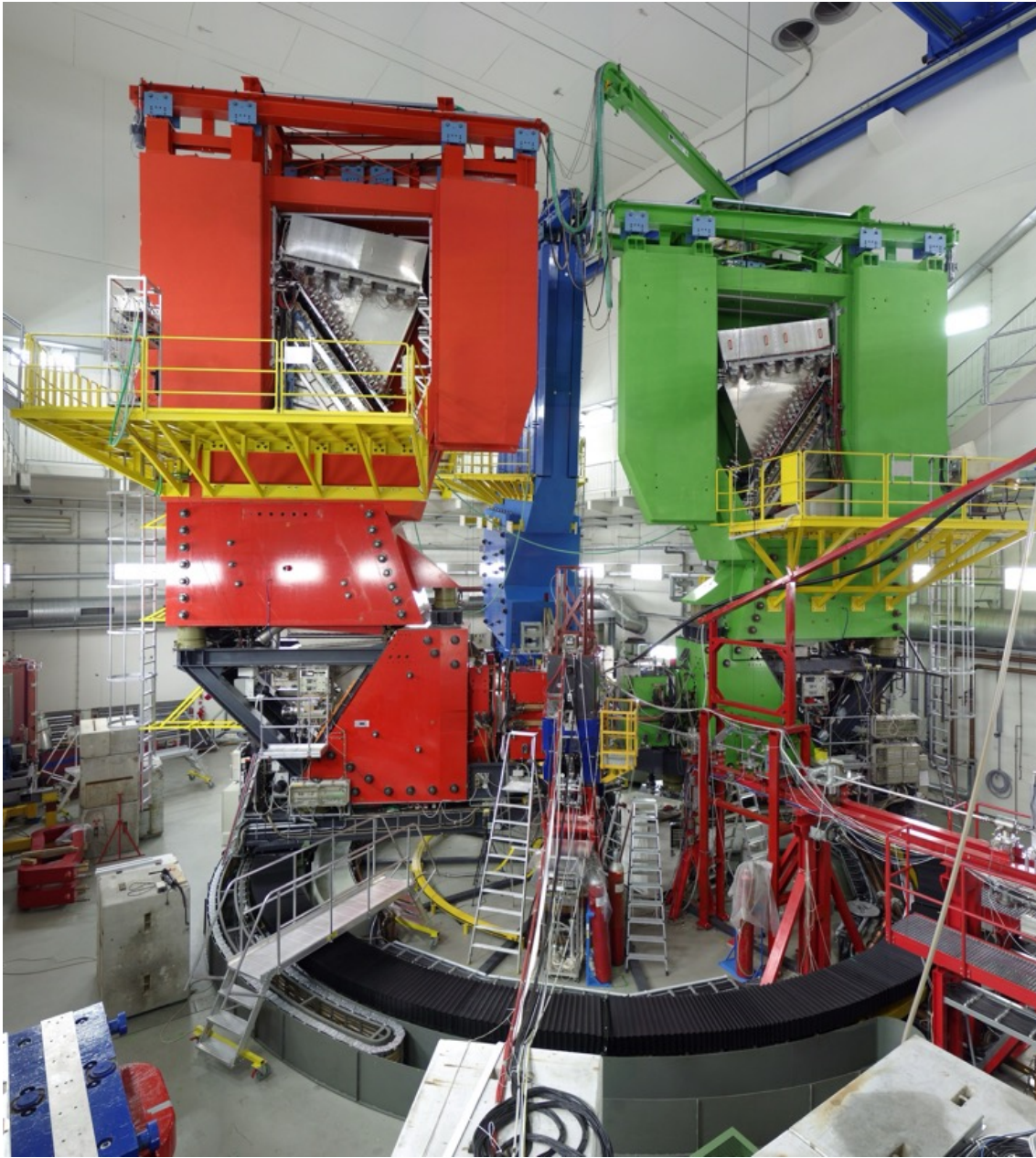
Figure 2.4: Picture of the A1 hall [Ber10]. From the left side, Spectrometer A (Spek-A, red one), Spectrometer B (Spek-B, blue one), and Spectrometer C (Spek-C, green one). These three vertical bending spectrometers are installed on the rolling stage. The radiation shielding doors of Spek-A and Spek-C are open in this picture.
